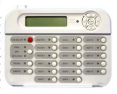
Shown below is a labeled remote control to a Pro Logic PS pool control. Note that labels have been placed over the generic names to make the keys human readable. In this case, the Pool Filter, Gas Heater, Spa Filter and Water Feature are all turned on.
