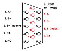
Solder side DB15-Male mating connector on cable and DB15-Female socket side at the SD1, SD3 & ACDC.
