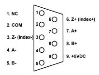
Solder side DB9-Male mating connector on cable and DB9-Female socket side at the CPU7, CPU10 or MPU11 connector.
