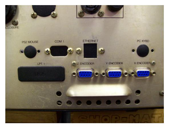
**Note:** If your system uses the COM port for the spindle speed control, instead of installing the blank out cover for COM1, install the RS-232 COM port cable to the back of the M15 back panel.
