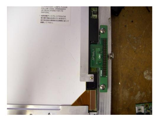
7. Install the bracket to secure the LCD cable connector to the connector on the LCD as shown in the picture below.
