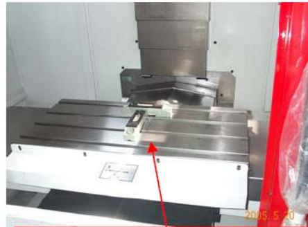
Figure 1.3, Move table all the way to the "front" and level in left and right direction.
