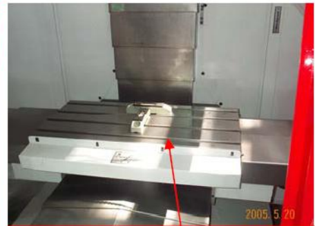
Figure 1.4, Move table all the way to the "back" and level in left and right direction.
