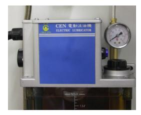
These pumps are designed to be operated exclusively with the Centroid control. The same guidlines for parameter 179 as listed above should be followed with this model pump.
