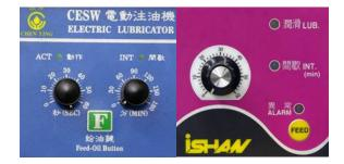
The interval (INT) timer should be set to 0 in all cases. When power is applied to the lubrication pump, the interval (INT) timer dictates when the pump will start running. For example, if the interval (INT) is set to 30, the pump will start running 30 minutes after power is applied. The control will only apply power to the lubrication pump for 15 sec. every 30 min. If this is set to anything other than 0, when power is applied the pump will never be activated.
