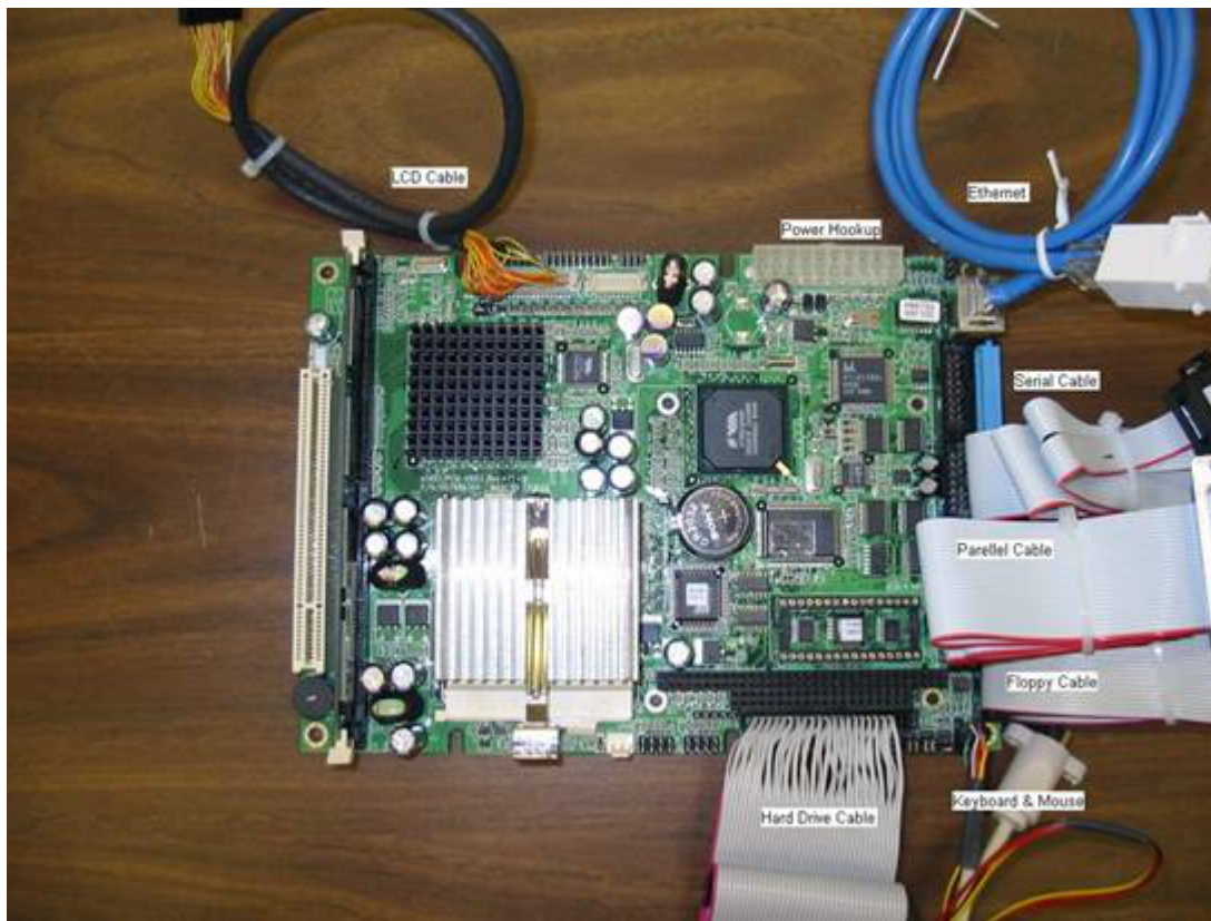
Picture 3: Aaeon with cables inserted correctly
