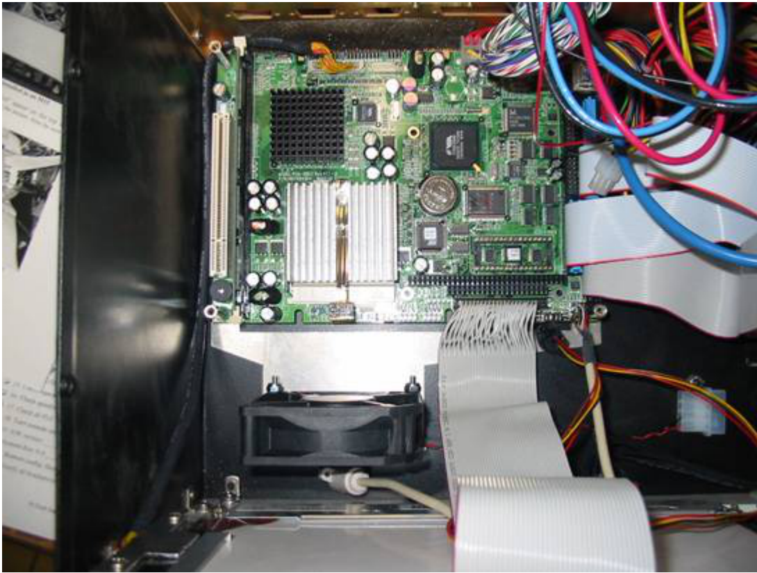
Picture 2: Aaeon motherboard installed in an M15
