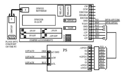
Or connect the Cosel PS and Spin232 (rev. C) according to this diagram.
